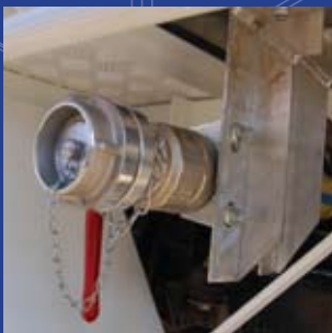
38mm Standpipe Side Fill.
